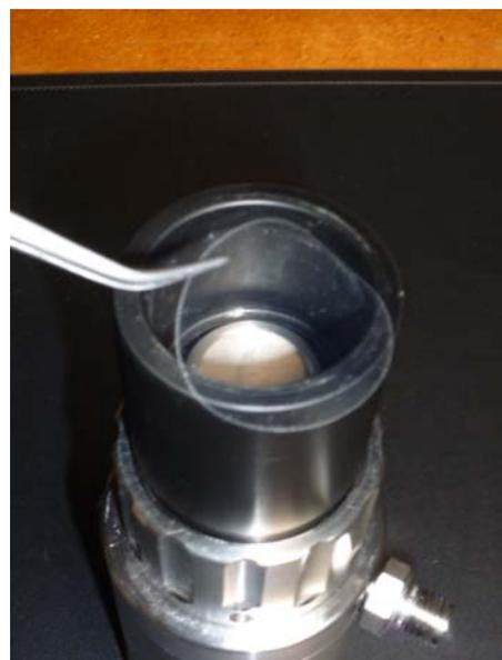
The membrane should be evenly spaced, centrally within the support.
