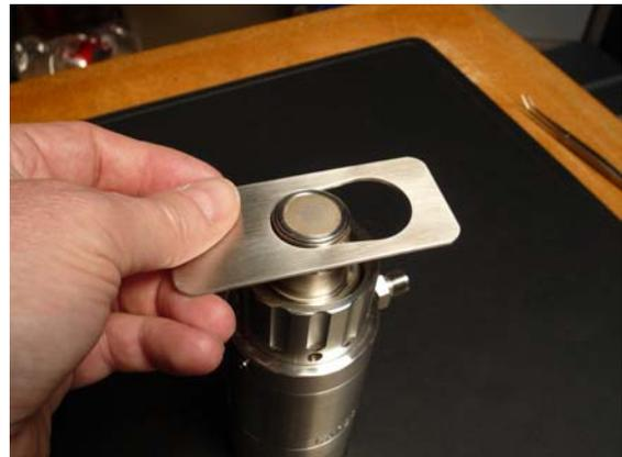
Now just lift the removal tool and the membrane and tightening ring will come free. Take care that the protective pastille remains in place (it can fall out). If it does fall out, simply replace it with great care – **DO NOT TOUCH** the chip. It is extremely delicate and easily damaged. Remove the old membrane to reveal the stainless steel grill in the sensing face.
